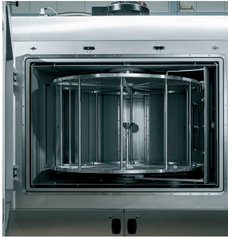
Flexible drum carrier with usable coating area up to 2.2m 2
