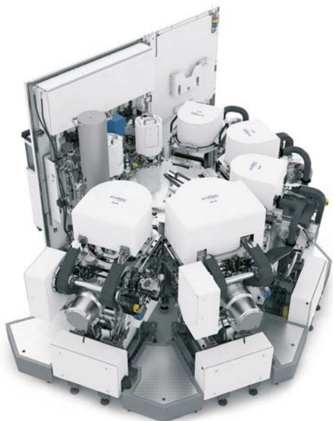
Figure 1a: CLUSTERLINE® 200 equipped with single process modules and FOUP
