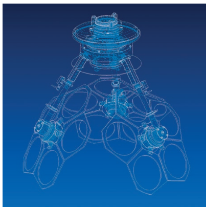
Flip system for double-sided coating
