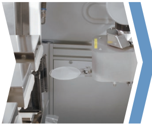
2. Precise handling of wafer by robot, including wafer centering.
