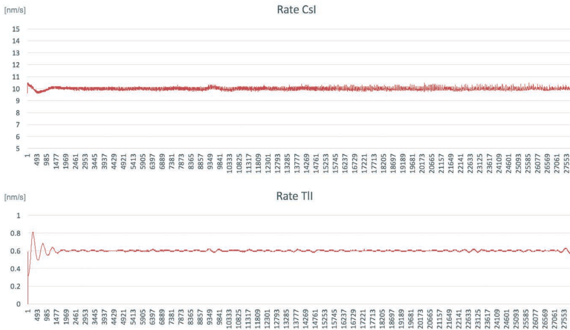
Controlled rates for CsI and TlI during the entire deposition of 7 hours
