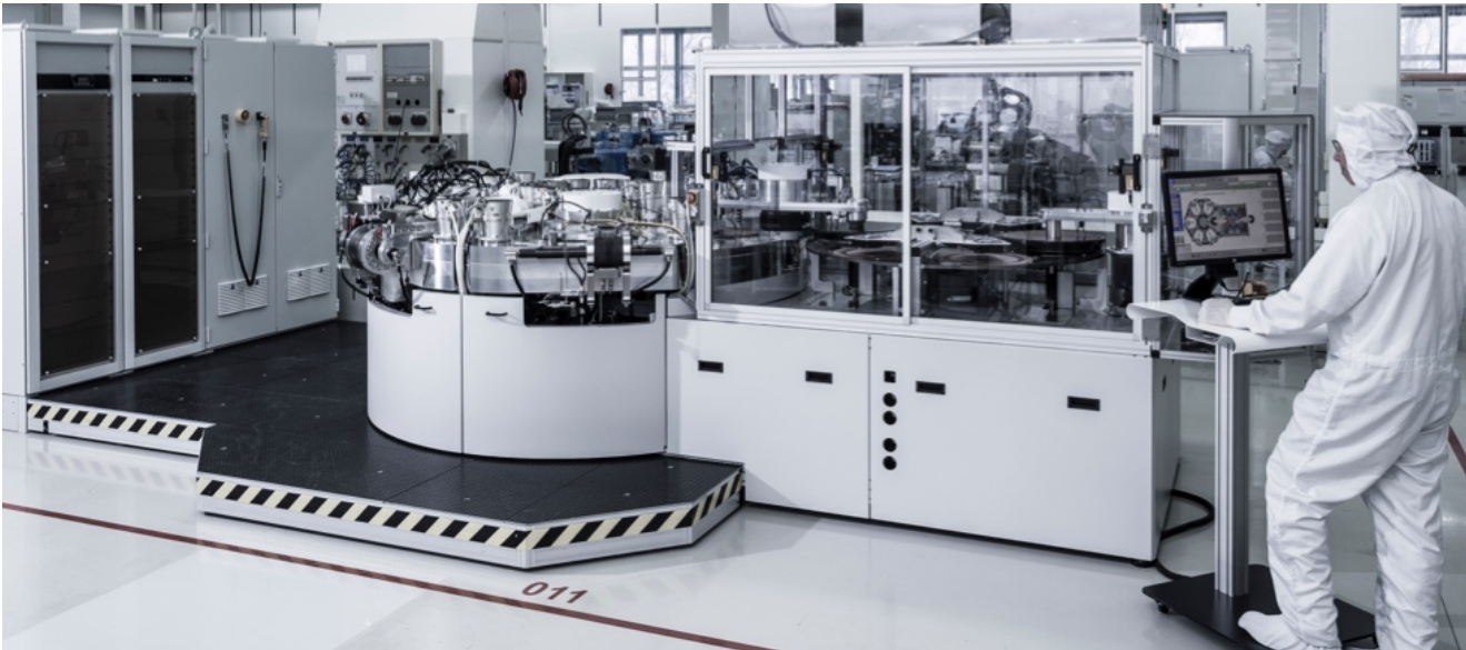
Fig 5: SOLARIS S380 high throughput inline sputter system
